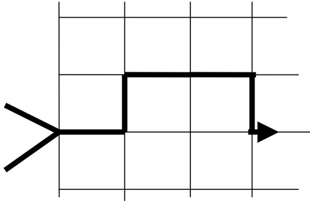
Figure 1. Crack growth in a lattice with randomized properties (scheme).
