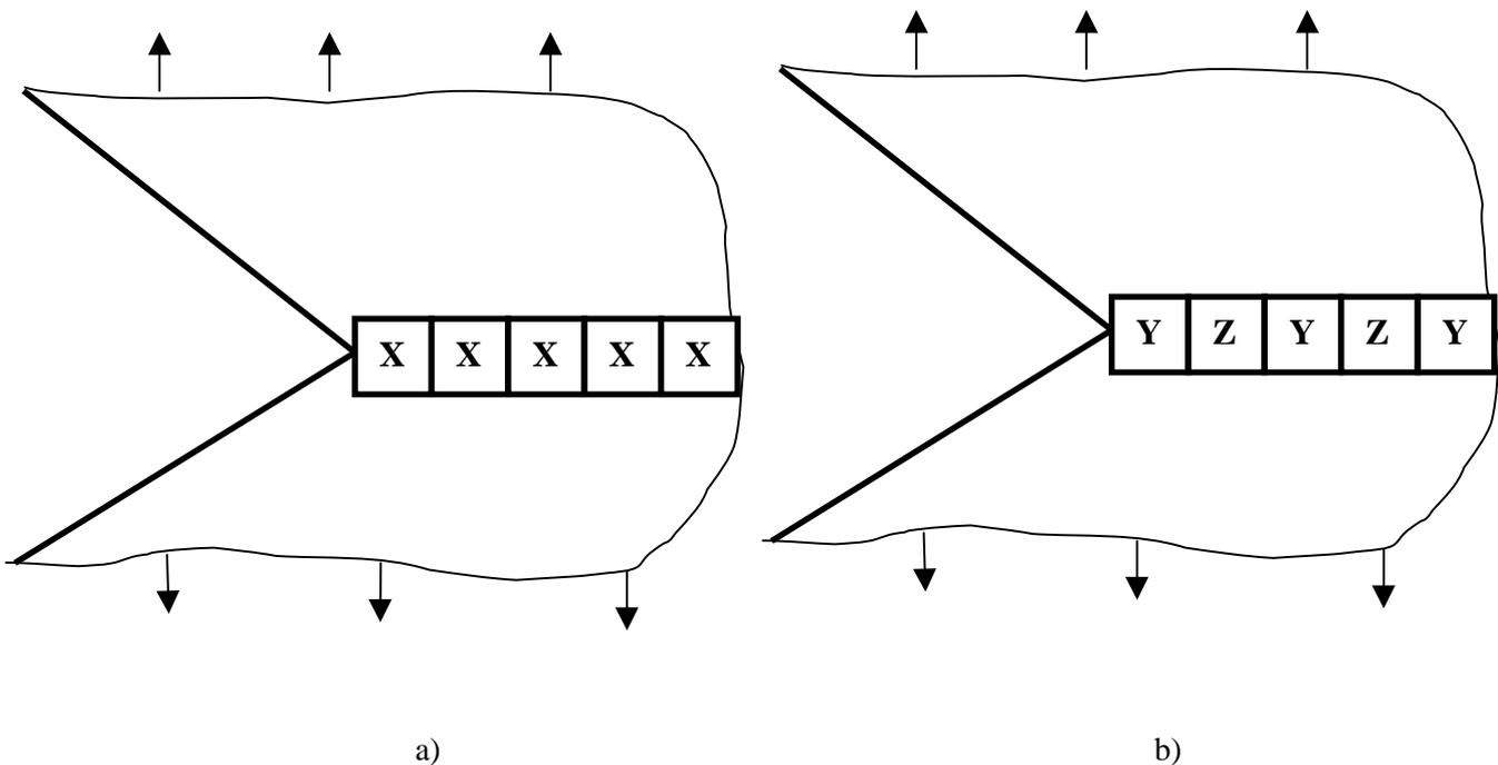
Figure 3. Crack growth in a homogeneous material (a) (phase X) and in a heterogeneous materials (b), phases Y and Z (scheme).
