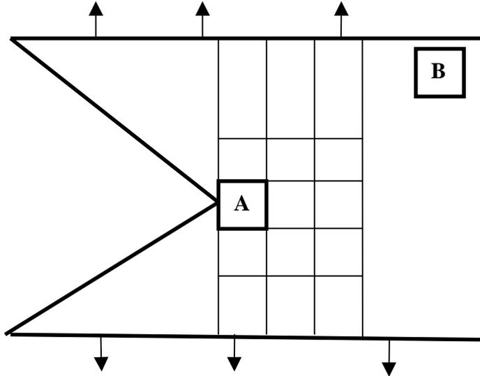
Figure 2. Initiation of microcracks in front of a growing crack (cell A) and in a random site (cell B) (scheme).
